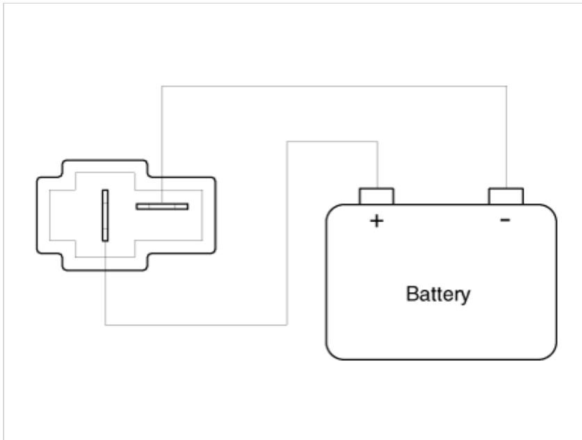
2. If the blower motor does not operate well, substitute with a known-good blower motor and check for proper operation.
